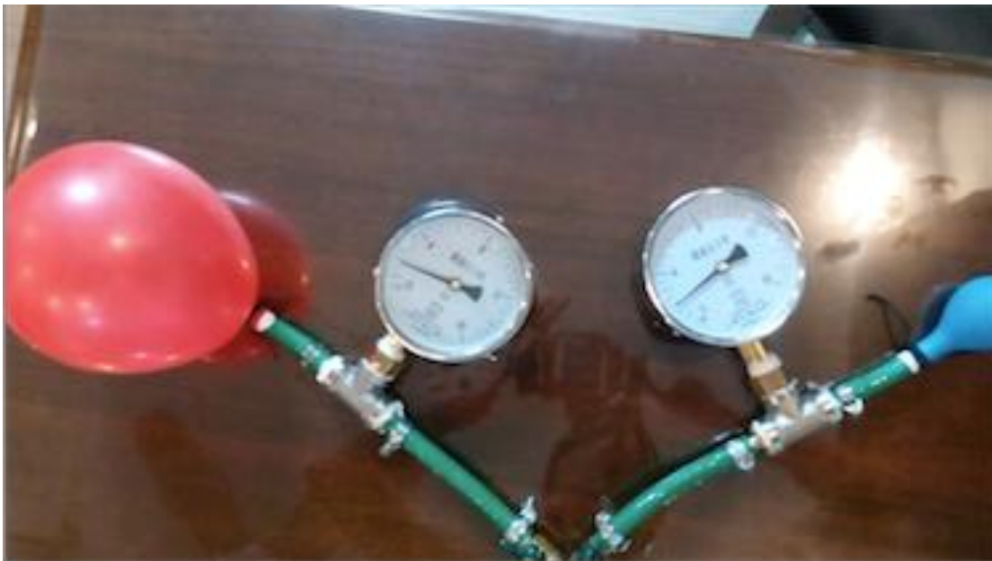
Pic 2. The small balloon shrinks almost to initial volume while big balloon expands. The difference in volumes increases.
